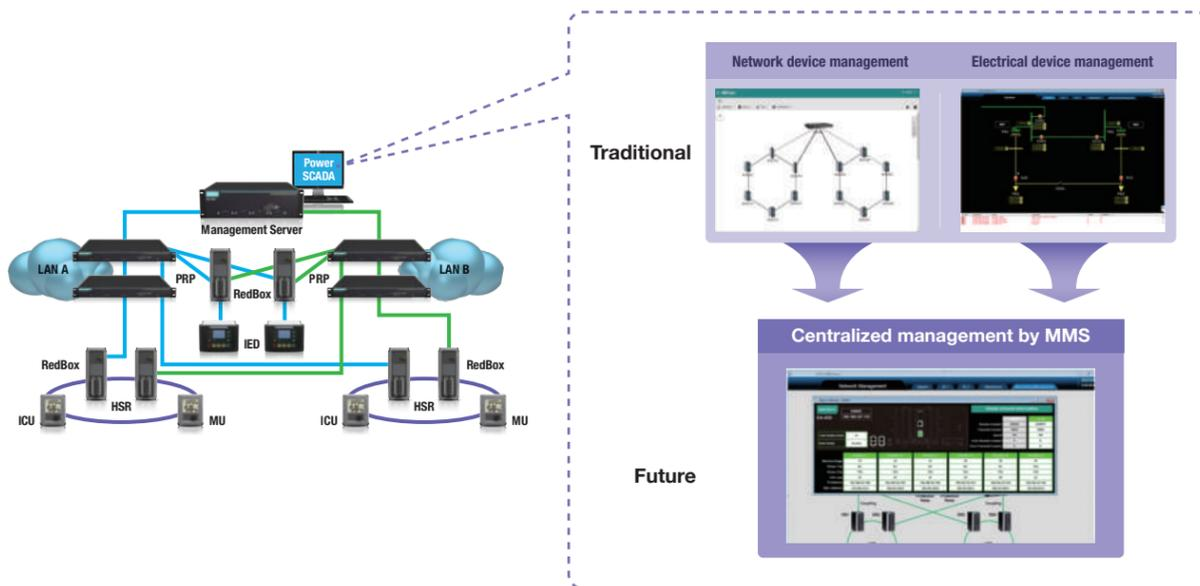
Sometimes substation networks deploy switches that do not have integrated IEC 61850 MMS, making network management more complex as these switches cannot be integrated easily into the PSCADA system. Moxa's network management software supports RESTful APIs and web widgets that enable easy integration of such devices with third-party applications (e.g., web-based SCADA).
