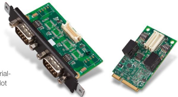
With over thirty years of experience in multiport serial board technology and development, Moxa can offer one of the most comprehensive selections of industrial-grade multiport serial cards on the market. We offer serial boards for a variety of slot types, from PCI, PCI Express (PCIe), PC/104 to mini-PCIe.
